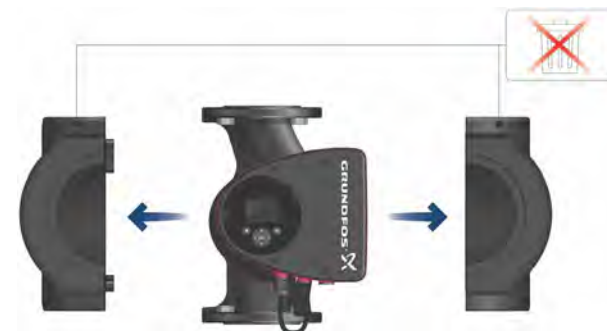
Fig. 3 Fitting insulating shells to the pump
