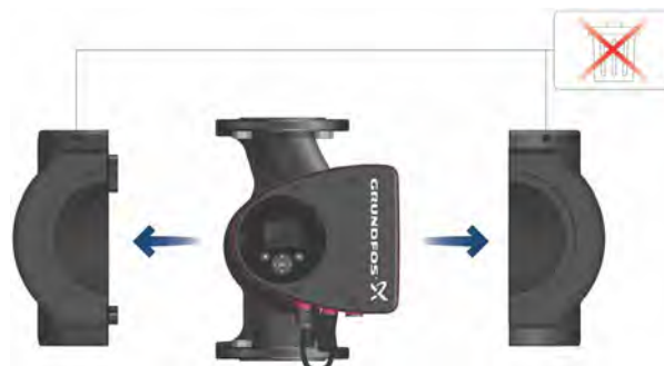
Fig. 3 Fitting insulating shells to the pump
