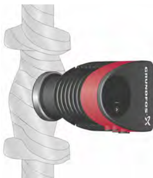
Fig. 13 Insulation of pump housing and pipework
