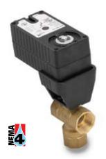
Three-way valve coil and bypass streams flow simultaneously through the ball. Bypass Cv is always 80% of coil Cv so there is always enough pressure drop in bypass mode. Three-way overflow problems are eliminated.
