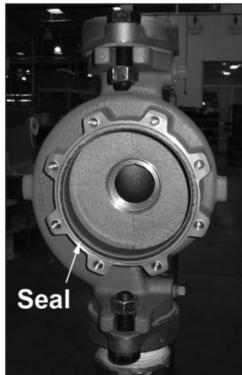
Fig. 37: Be sure not to damage the seal when removing or replacing the pump body
