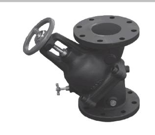
Grundfos Series CV, Combination valve combines three valves in one: shut-off valve, balancing valve, and check valve. The combination valve makes it possible to reduce the overall system pressure drop since fewer individual components are needed when installing a pump.
